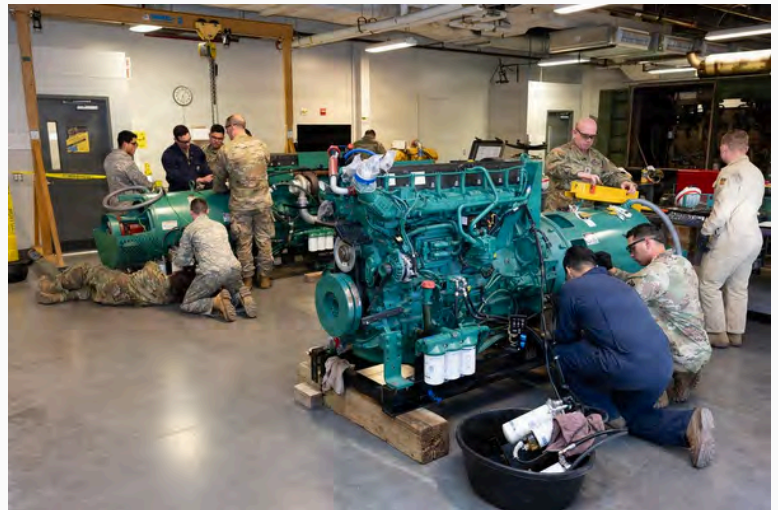
U.S. Army Prime Power School Advanced Leader Course students practice splitting and reconnecting power packs Feb. 23 at Fort Leonard Wood.
